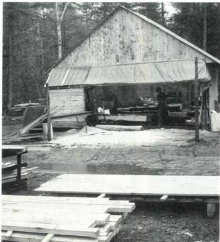
A covered sawing station keeps out the rain for Dennis and his Ross bandmill.
