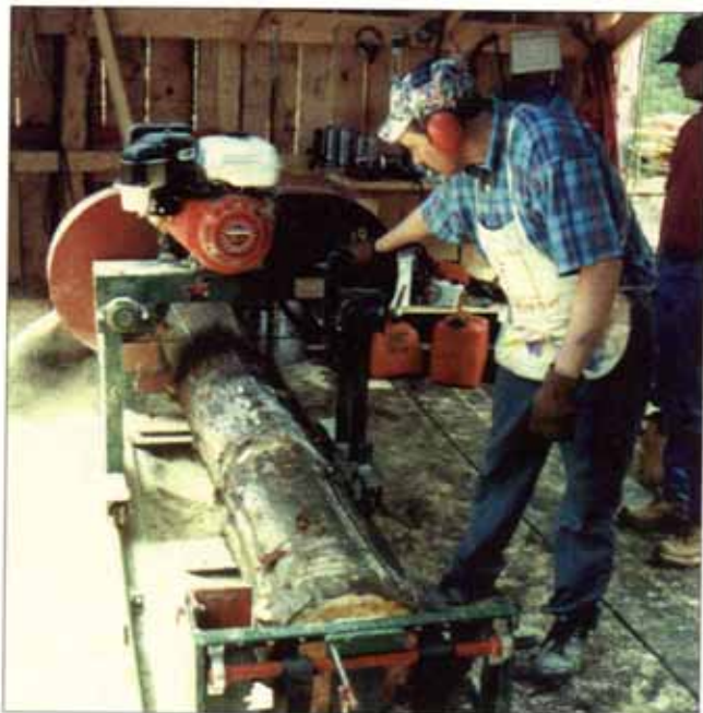
The Ross saw head is light enough to push easily.
