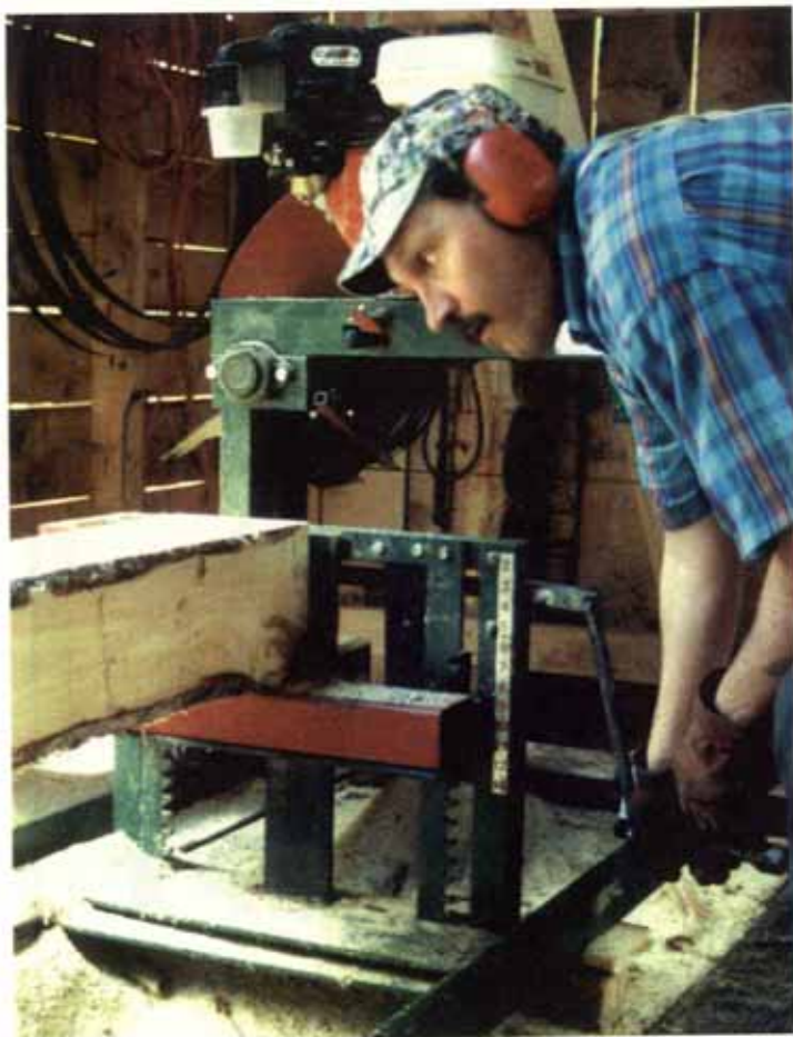
Dennis Martin cranks up the log for his next cut. Note the 2-inch spacer used to set taper.
