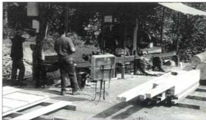
Joe Slater mills recycled logs into packaging timber and framing lumber.
