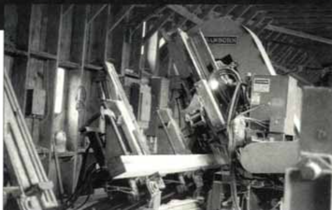
The headblock/knee assembly on the Min-Max shows the top and bottom dogs. The taper adjustments are on the opposite side of the knees.
