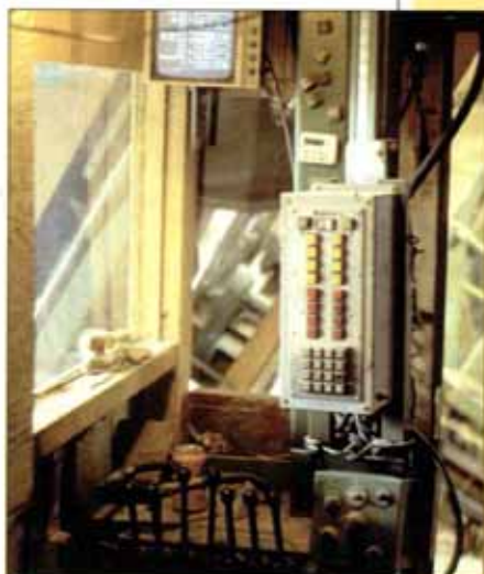
The sawyer's work station, showing all the handles and buttons along with the display for the computerized networks.
