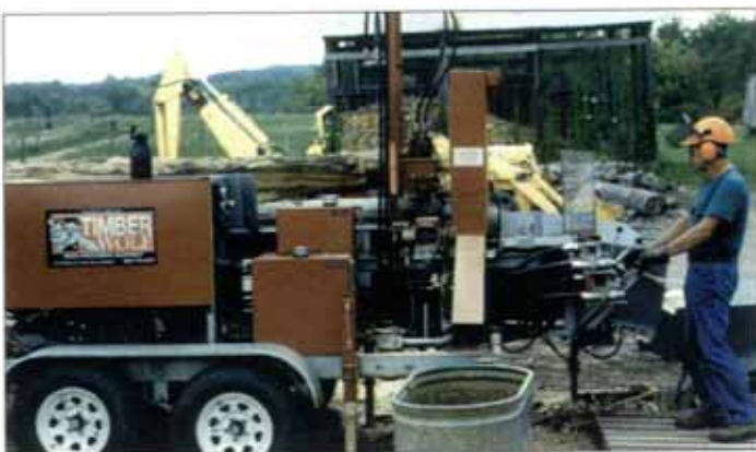
With the operator controls near the splitting trough, it's easy to position logs.
