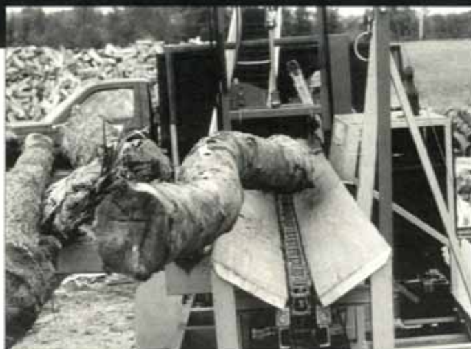
The top roll makes it easier to handle crooked logs.
