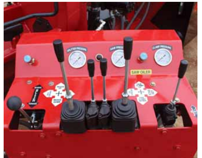
The controls are simple, with all levers on a dead-man switch for safety.
