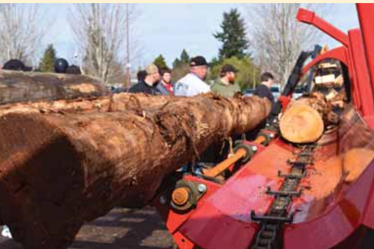
The rounded log trough allows the operator to feed in misshapen logs that might otherwise be considered worthless.
