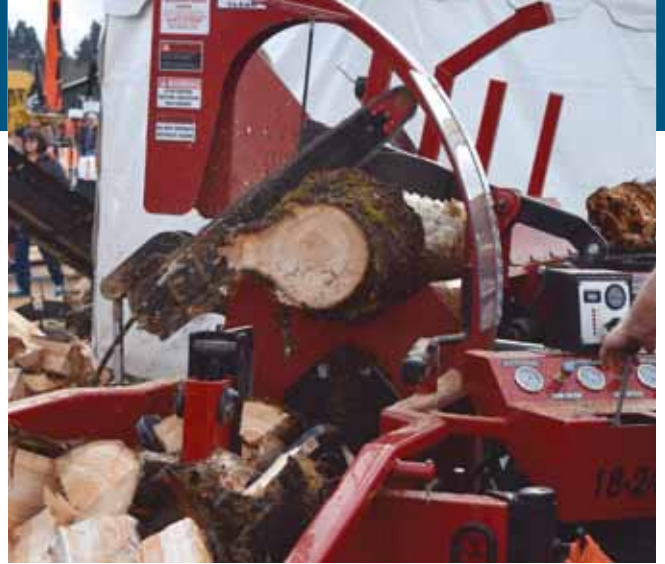
At the far end of the rounded log trough, the clamp (right) descends to grip the log. A pressure-sensitive connection then engages the chain saw blade (left), which makes the cut. When the blade is raised, the action is reversed.
