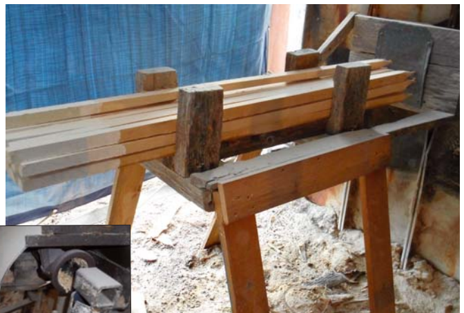
After sharpening, stakes are fitted into a jig that holds 25 stakes that are then tied with wire to form a tight bundle. The stake pointer was salvaged from the fire, but has a new motor (inset left).
