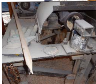
After sharpening, stakes are fitted into a jig that holds 25 stakes that are then tied with wire to form a tight bundle. The stake pointer was salvaged from the fire, but has a new motor (inset left).
