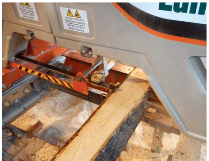
When sawing small logs, the right-side blade guide can be positioned close to the log to minimize blade deflection.
