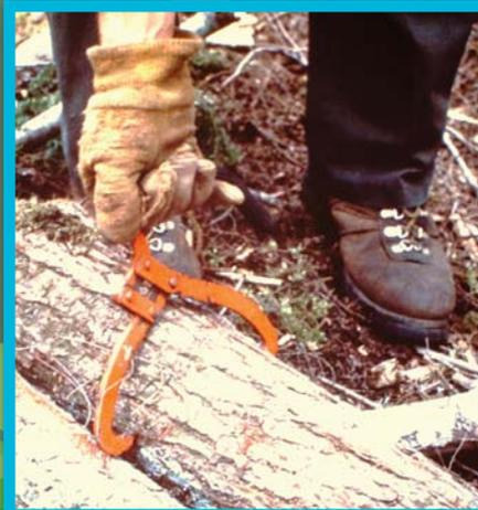
Photo 1. Hand tongs facilitate lifting and moving wood. They reduce bending and provide a good grip on logs, bolts, or trees.
