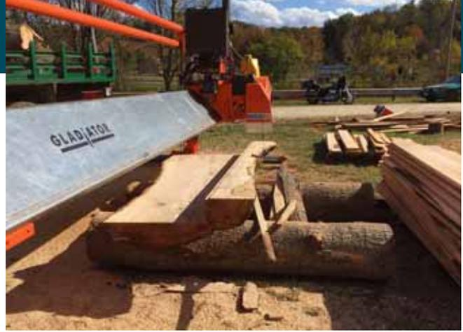
The TurboSawmill Gladiator takes a bite out of a log. With a 12-inch cutting depth and a 46-hp Kubota diesel engine, it can not only handle large logs but produce wide boards and beams up to 12 inches by 24 inches (by using the double-cut technique).
