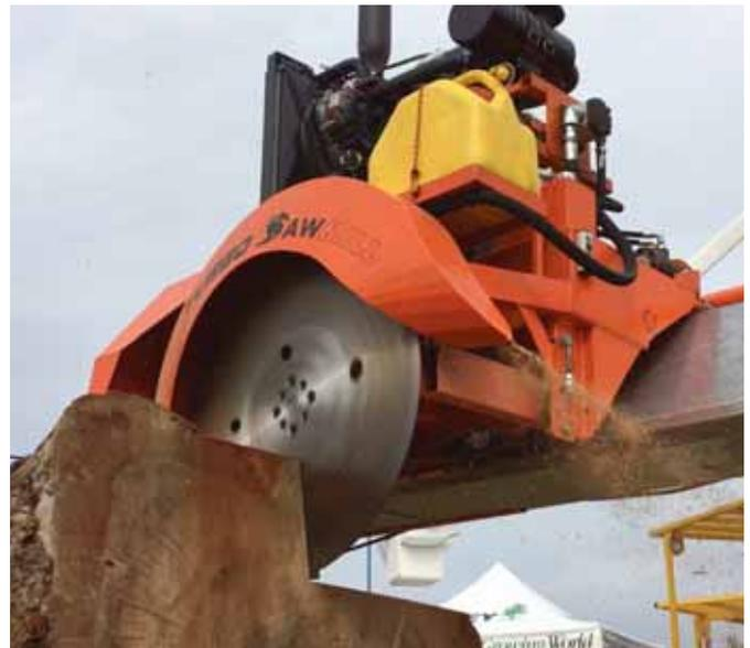
With a 33-inch-diameter blade and a 46-hp Kubota diesel engine, the TurboSaw Gladiator can take on logs of nearly any diameter. The single rail provides a rigid support for the sawhead, and avoids any issues with the log fitting inside a frame.
