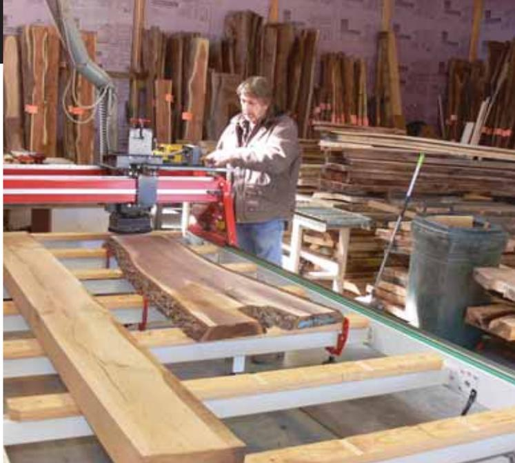
One more pass should just about get it! Kerry sets up the Wood Wizz for its next pass. Once the entire slab is flattened, he'll make a thin skimming cut to clean up the surface.
