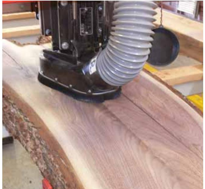
The Wood Wizz has a 5-inch cutting width and 1/8-inch cutting depth, leaving a smooth, flat surface on this walnut slab.
