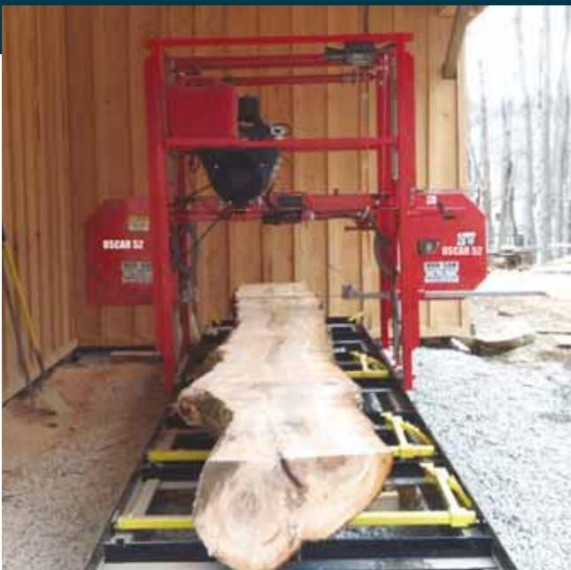
With a 48-in. width cutting capacity, the Oscar 52 has no problem slabbing irregular shapes, allowing the sawyer to make unique lumber available to woodworking customers.
