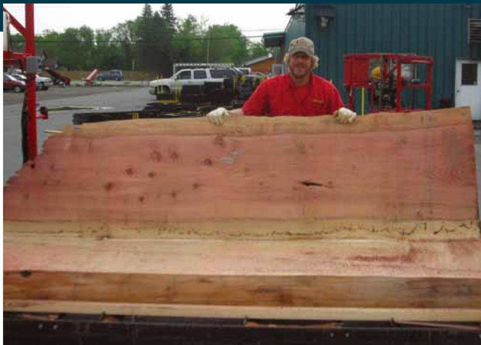
Wide slabs are currently in high demand by woodworkers. Ken shows off a 32-in. wide slab freshly cut by his Oscar 52. The 2-in. thick slab will air-dry for a year before going into a kiln for final drying.
