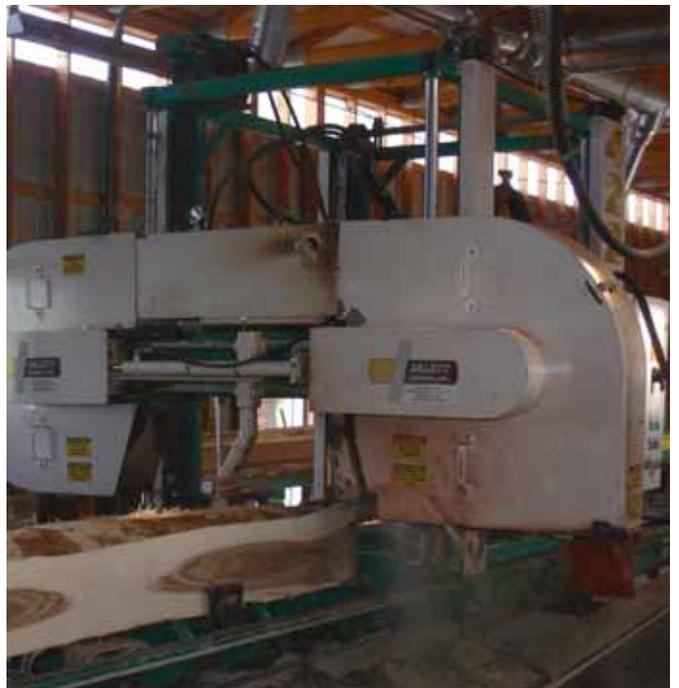
The unique bi-directional cutting action of the Select mill, coupled with a feed rate of up to 3 feet per second, makes for high production. Frequent turning to the best face maximizes the quality of the lumber.
