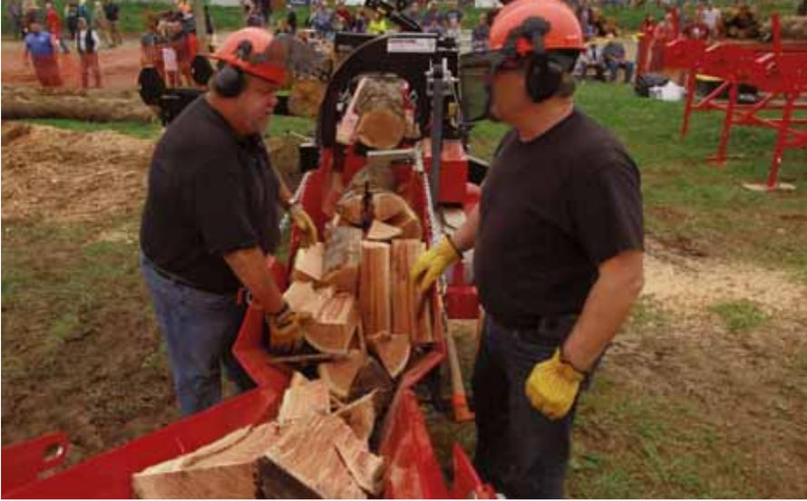
outfeed conveyor slipped. “We should have tensioned it before the Shoot-Out,” Scott admitted. In a few minutes, he and Bryndon had everything back on track, and the 12-foot conveyor was dumping the wood in a neat pile as fast as Scott and Bryndon could cut and split it. The machine performed right in the middle of the 2 to 3 cords per hour that Wood Beaver claims for this machine. He says he knew that the Wood
