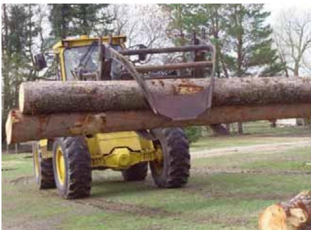
Spruce logs are among the most difficult logs to saw on a band saw mill because they have soft wood and hard knots that can result in wavy lumber.
