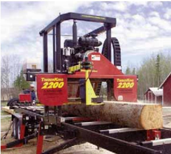
Hydraulics, board return and debarker were important features when Gary Francis went shopping for a new band saw. He got it with the TimberKing 2200. These features reduce his back pain and minimize the potential for grit, which is deadly to band saw mill blades.
