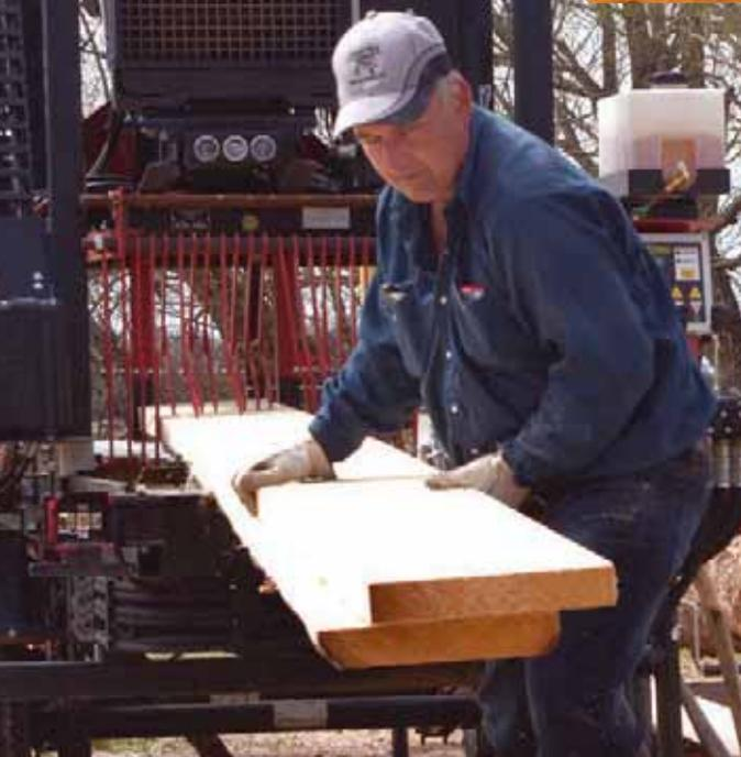
Gary Francis says that he can manufacture about 800 board feet of lumber per hour using his TimberKing 2200 band saw mill.
