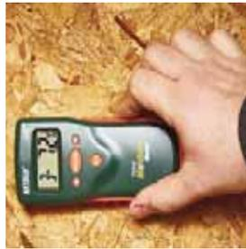
Special note: Older moisture meters were often designed for use with a four-pin probe. The readings with two pins in a four-pin meter are 1/2% to 1% lower.
