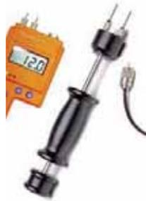
then pieces within the load can be measured for MC. Although the accuracy is not high, this probe can detect the wetter pieces, such as when air-dried lumber is going into a kiln. The wettest pieces are chosen for samples during the run.
