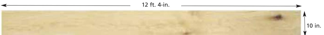
Example 2 of calculating board feet: A board 10 inches wide and 12 feet 4 inches long is 8/4-inch thickness has how many board feet?..... $10 \times 12 / 12 = SM$  of 10;  $10 \times 2$  inches = 20 board feet.
