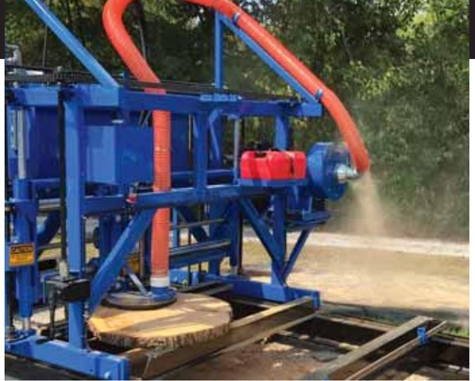
The surfacing unit has both a rotary cutterhead and a coarse sander that can handle both conventional slabs and “cookies.”
