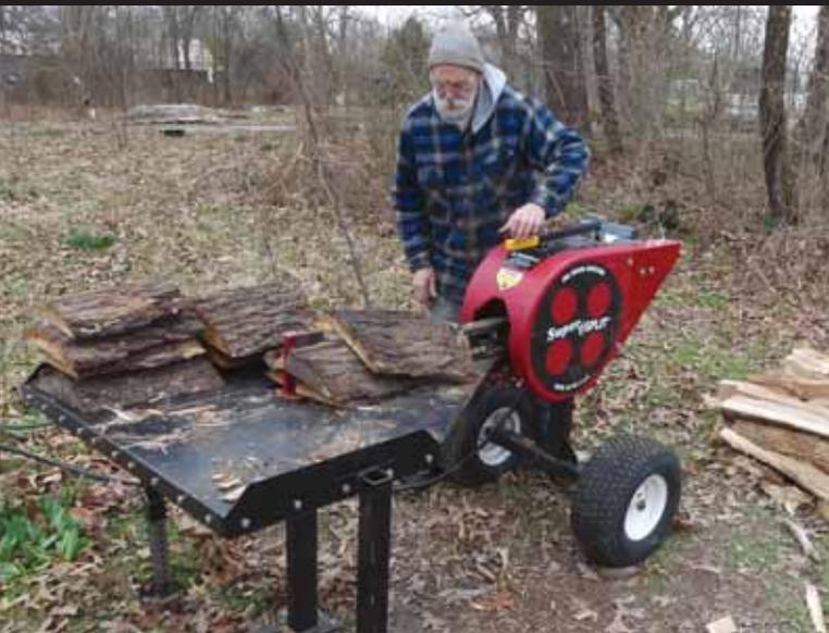
The three-second cycle time of the SuperSplit kinetic splitter is especially useful in splitting firewood slabs, which may provide an additional source of income to small sawmills.
