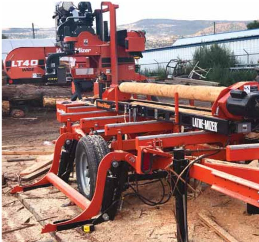
The Lathe-Mizer accessory allows Valley View Industries to produce round, hexagon-, octagon-, and triangle-shaped logs for building projects.
