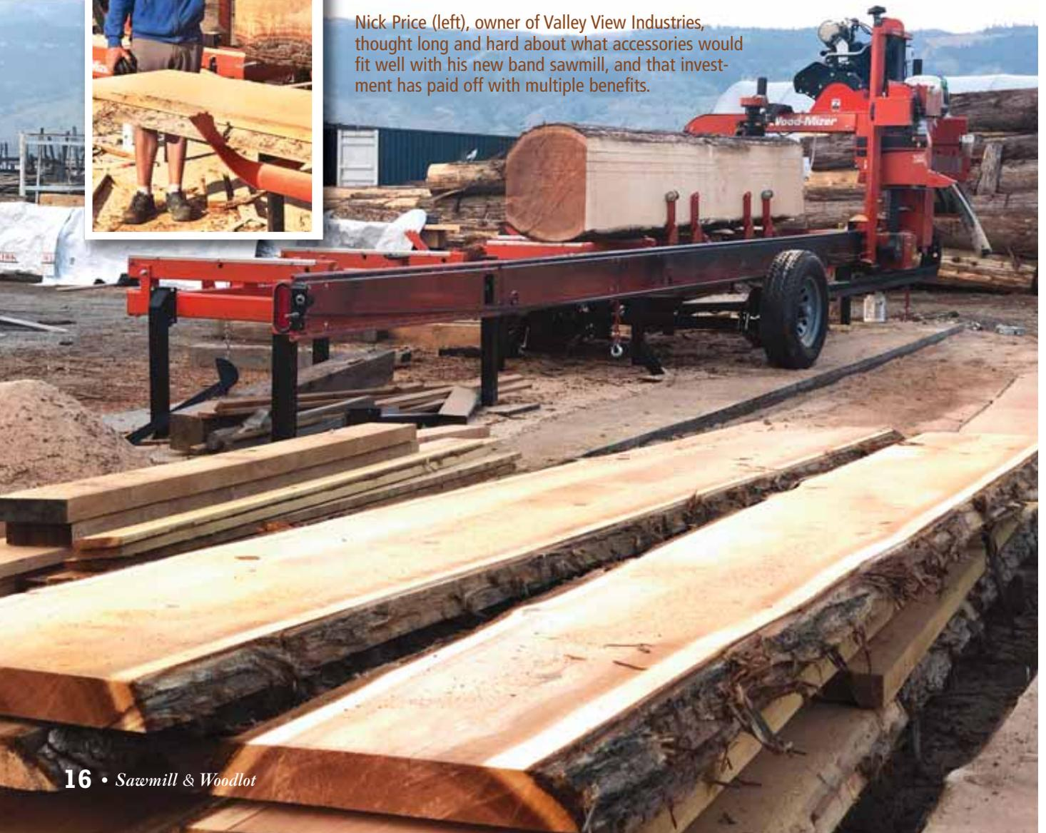
While they chose a Wood-Mizer LT40 band sawmill as their main breakdown unit, they also purchased a bed extension, debarker add-on, twin-blade edger, 4-sided planer/moulder, and Wood-Mizer's Lathe-Mizer tenon kit.
