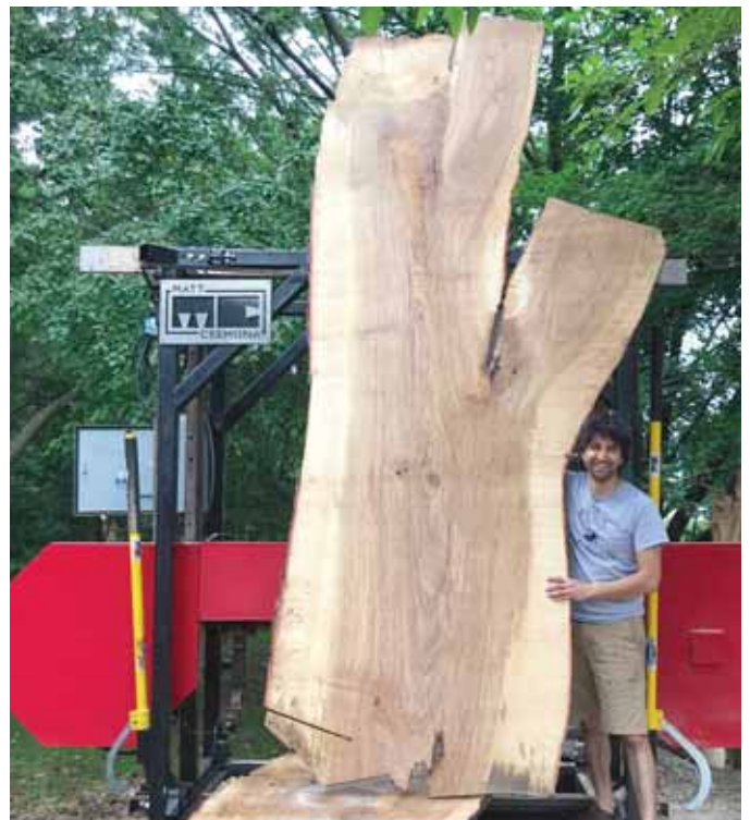
Above: Milling a big maple log on the mill. The 30-inch band wheels allow a throat for up to an 18-inch depth of cut. Right: Even the six-foot capacity of Matt's sawmill gets pushed to the limit cutting slabs like this one. The machine is designed to allow Matt to mill logs no other local mill can handle. His ships his slabs to woodworkers all over North America.
