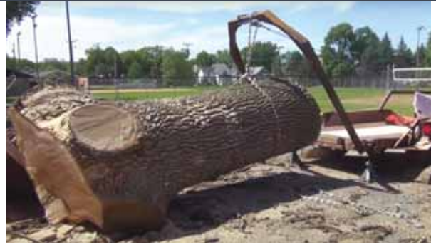
A trailer with a pivoting arch on a winch make picking up this huge ash log a piece of cake.
