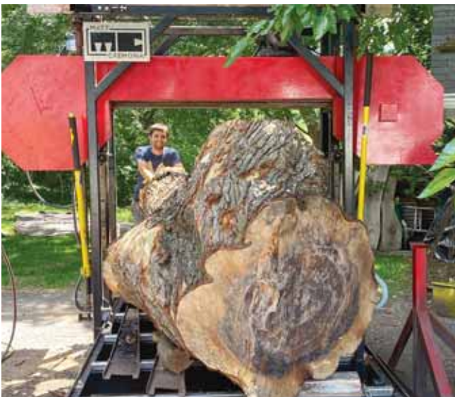
Above: Milling a big maple log on the mill. The 30-inch band wheels allow a throat for up to an 18-inch depth of cut. Right: Even the six-foot capacity of Matt's sawmill gets pushed to the limit cutting slabs like this one. The machine is designed to allow Matt to mill logs no other local mill can handle. His ships his slabs to woodworkers all over North America.
