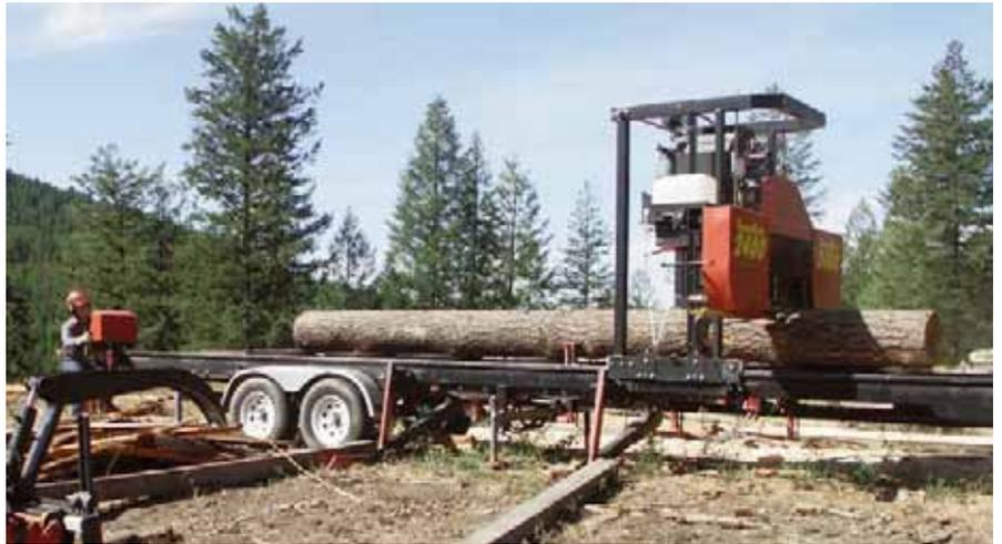
With the command post swung to the side for a better view, Bruce makes a slabbing cut for a beam. As a one-man operation, he says that he depends on the hydraulic log handling (lifting, turning, toe boards and clamping) capabilities of his mill.
