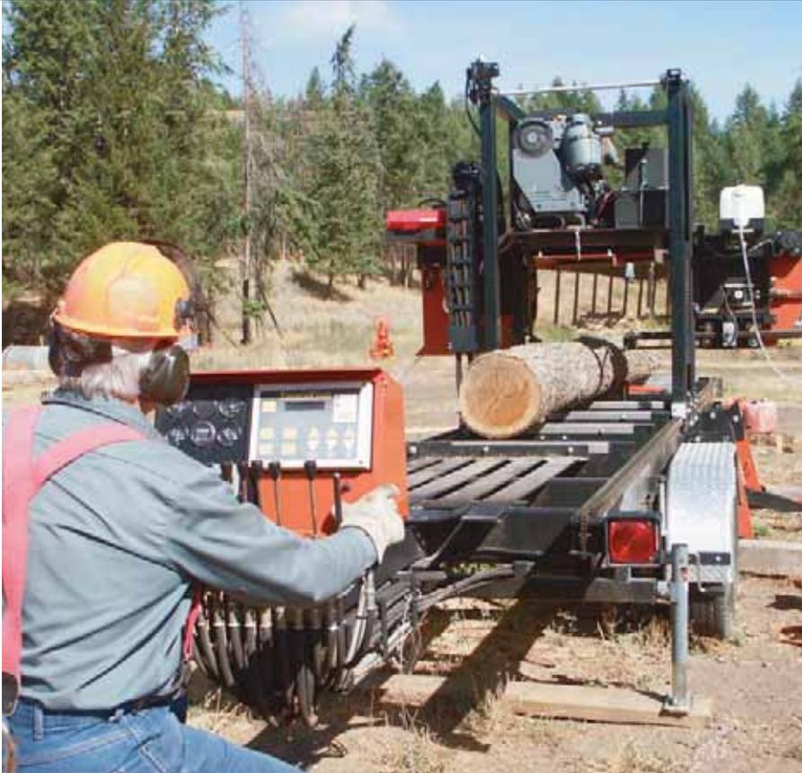
Sawyer's-eye view of the 2400. All hydraulics, electrical controls, and engine gauges are in the pivoting command post. According to Bruce, the mill's design and heavy construction allow him to exceed his customers' requirements for straight, smooth beams.
