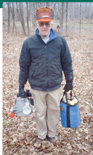
The PW is extremely portable. One man can easily carry the winch, rope, and accessories into the stand.
