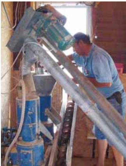
Mark adjusts a steam humidifier to get the desired moisture in the wood. His two pellet mills run off the PTO shaft (lower left in the photo) of his 150-hp Deutz tractor. The two angled pipes transfer the wood flour from the hopper to the pellet mills and the open auger transfers the pellets to a grain cleaner to remove the dust.
