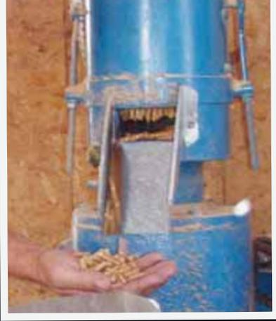
**Left:** Mark checks the flow of wood flour into his mills. He salvaged the augers and 3-phase motors from a junkyard, and added a variable speed control so that he could control them independently.
