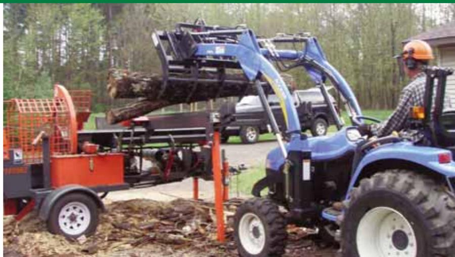
Larry Hanke uses his tractor with a grapple loader to set poles on the processor's live deck. According to Larry, the live deck arrangement works well for his operation, and has stood up well to having all sizes of logs dropped onto it.
