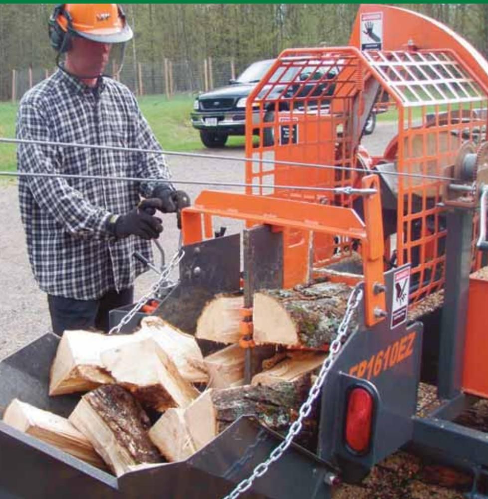
The 4-way wedge slides to evenly split different-diameter logs. In the up or down position, it acts as a 2-way splitter. Larry also keeps a 6-way wedge for larger logs.
