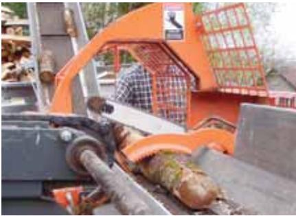
A view of the conveyer, clamp, and saw. The machine operated smoothly, and the only time Larry had to leave the operator's station was to help an occasional log off the live deck onto the conveyer.
