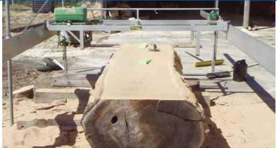
Above: Partway through slabbing a 37-in.-diameter red oak log. Below: The Lucas Model 8 Slabber utilizes a 66-in. saw bar and 190-link super skip ripping edge.
