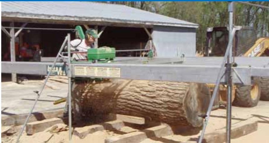
The framework and outrigger supports provide a stable platform for slabbing even the largest logs.
