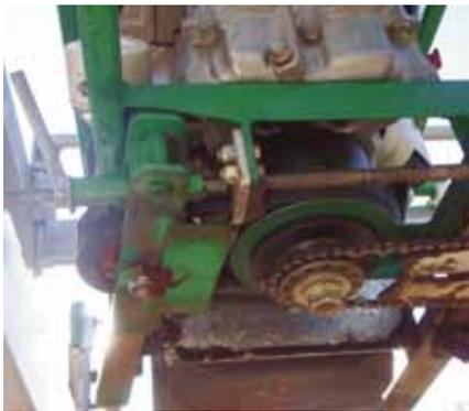
The simple tension mechanism tightens both the v-belt and the chain.
