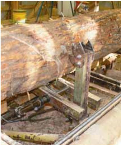
Jake's hydraulic log turner was made out of parts that he scrounged up and fabricated. The claw doubles as a log clamp.
