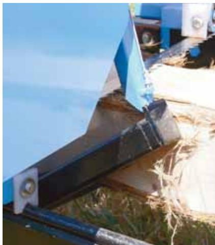
Close-up of the blade catcher that stops the forward movement of the carriage if the blade is low enough to hit a log stop.
