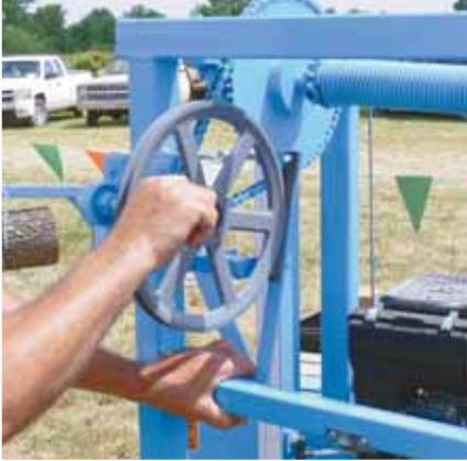
Ed Zimmerman demonstrates the EZ Boardwalk Jr. To set the carriage height, he releases the brake with his left hand while cranking with his right. The coil spring is designed to balance the weight of the engine and band wheels.
