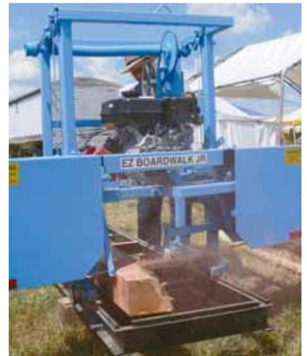
EZ Boardwalk designer Ed Zimmerman demonstrates the EZ boardwalk Jr. Notice the angle of the blade, which helps feed the mill through the wood.
