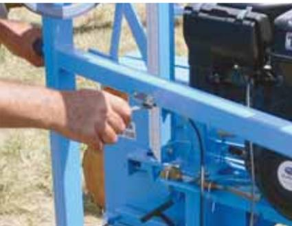
Frame-mounted throttle control is one of the new features of the mill based on customer suggestions.
