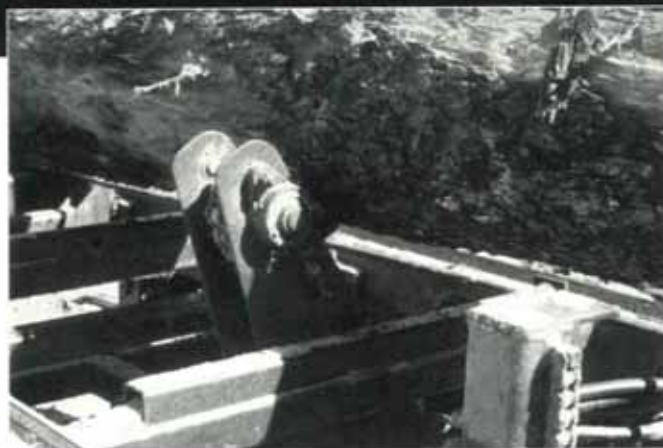
The chain-driven log turner has turnup/turndown capability.
