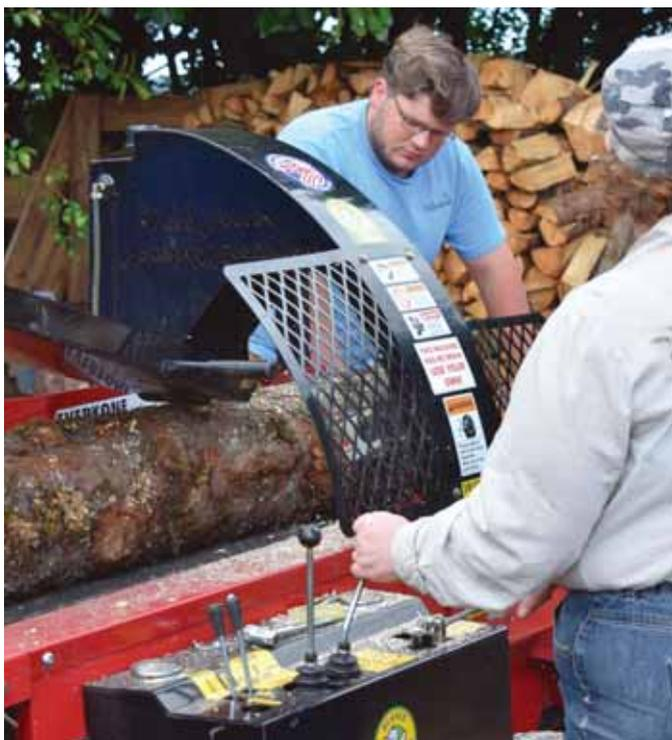
Becky Williams operates the Wood Beaver using a simple set of levers. Her son, Lee, lowers the protective lockout cover before engaging the saw and splitter.
