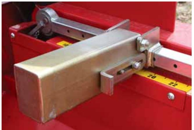
**By pulling the pin out, the log length adjuster can be set between 10 and 24 inches. Becky generally cuts her logs in 16-inch lengths, but can cut shorter for custom orders and smaller chimney-style firepits.**
