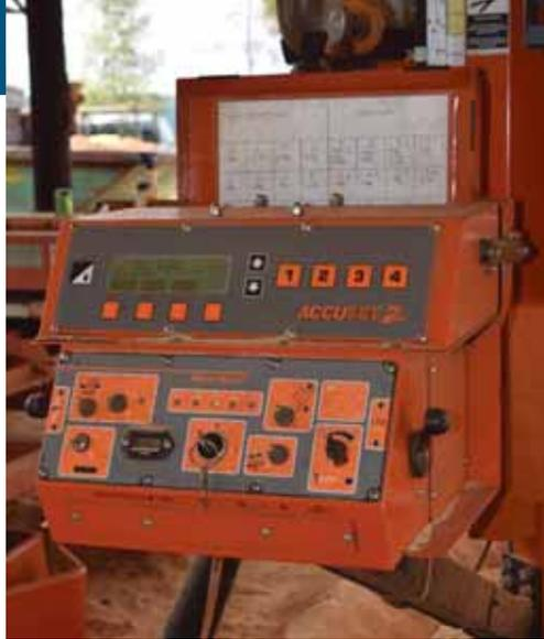
All log-handling functions are hydraulically driven and operated using Wood-Mizer's Accuset 2 computerized setworks to automatically calculate board thickness and move the sawhead into place for the next cut.
