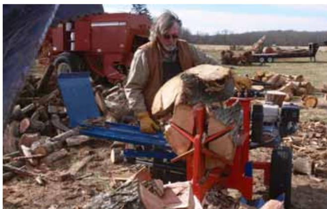
Once the initial splits were made, John raised the wedge for a 6-way split. The 12-hp Honda and 2-stage hydraulic pump had no problem crushing it way through this one.
