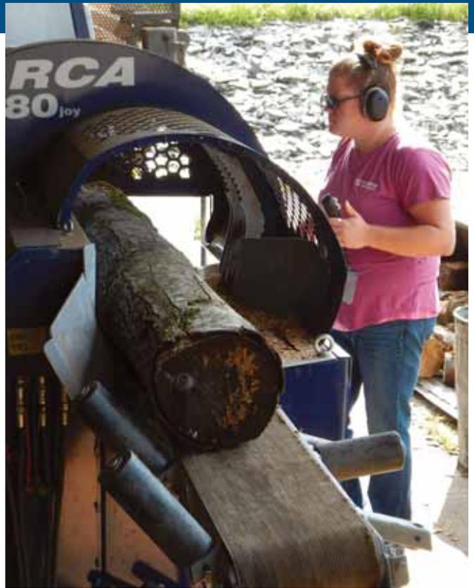
Jessica Perkins controls the splitting cycle of the Joy 480. She says that the simple joystick control makes the machine very easy to learn. The Joy 480 meets international safety standards. For example, opening the cover stops all mechanical functions.
