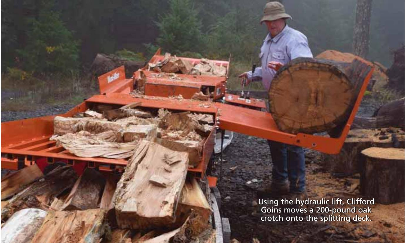
Using the hydraulic lift, Clifford Goins moves a 200-pound oak crotch onto the splitting deck.
