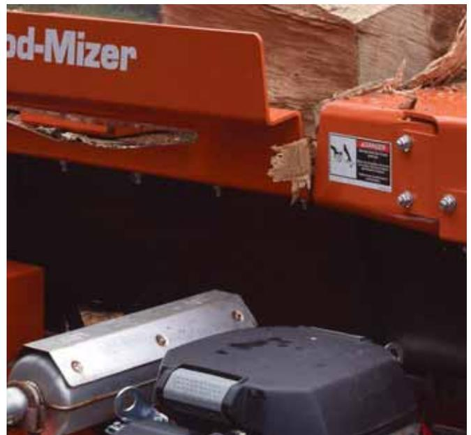
Goins’s only concern about the splitter was the buildup of chips and shavings in a gap in this guard. Wood-Mizer has already addressed the issue in new designs and is providing parts for current owners to retrofit.
