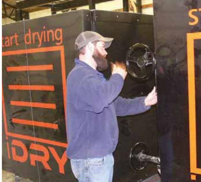
Loren Bates opens up a kiln to check a load of oak. The pressure inside the kiln is so great that a valve must be opened to equalize the pressure before the door can be opened.
