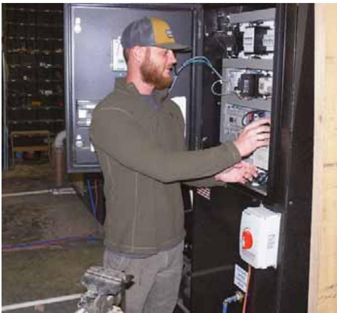
Jesse Lamborn shows the inner workings of the iDry kiln. According to Jesse, the automated unit pretty much runs itself once it has been loaded and the thickness of the wood has been entered.
