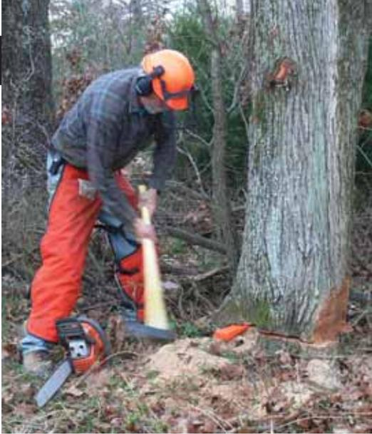
Left: If you suspect back lean on a tree, drive in a wedge behind the hinge to hold it off your saw while you finish the cut. Then drive in the wedge to topple the tree over (it may take several wedges).
