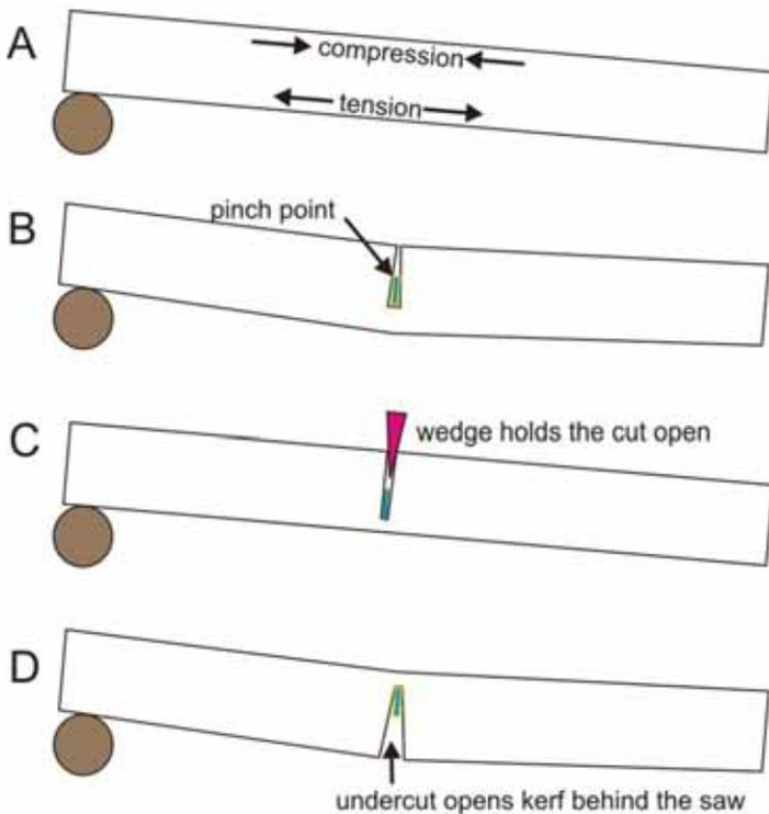
A simple beam is supported on both ends. Gravity puts the top of the beam under compression and the bottom in tension (A). These are equal but opposite forces. Cutting from the top results in compression against the chain saw bar, pinching it (B). Driving a logging wedge in the top (C) holds the compression off the bar, allowing you to finish the cut. Another strategy is to cut from the bottom up (D) allowing the tension to pull the cut open as you complete it.
