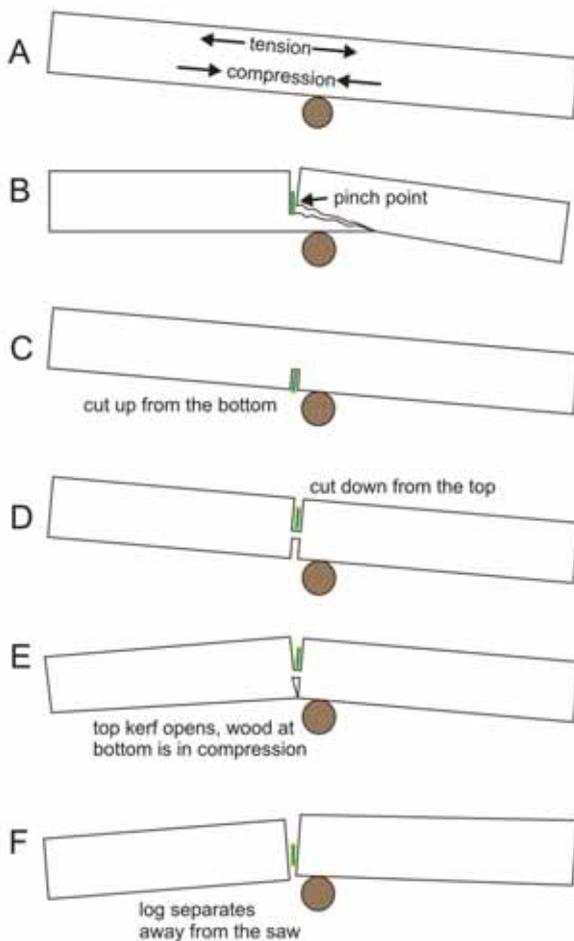
A cantilevered beam is supported on one end, putting the top in tension and the bottom under compression (A). Cutting from the top down relieves the tension as the fibers pull the cut open, but shear stress can cause the log to split, damaging the log and pinching your saw (B). Starting the cut from the bottom (C), then finishing the cut from the top (D), pulls the top kerf apart and compresses the bottom kerf (E), which pushes the log apart as you finish the cut (F).
