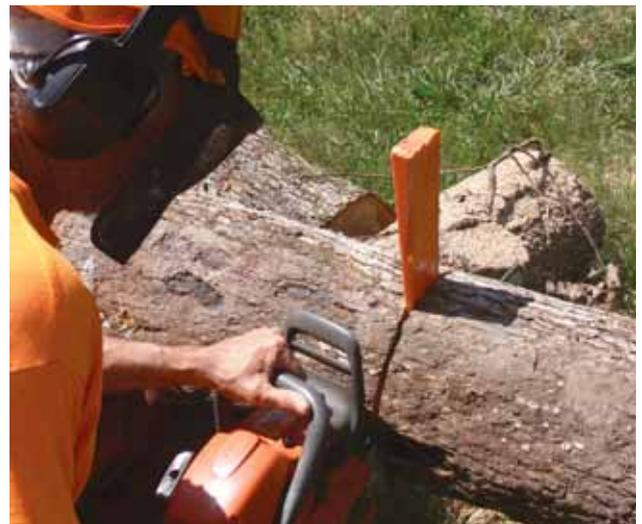
With the wedge in place, you can finish cutting a simple beam without pinching the bar.
