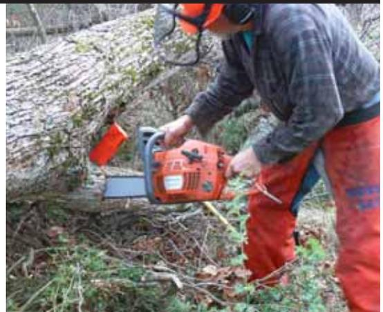
I bind up more bars when limbing than any other time. Limbs are often under torsion (twisting) as well as compression and tension. Cut 90 degrees to the branch and drive in a wedge to keep the pressure off the bar.
