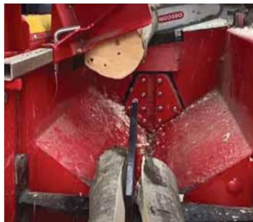
The cutoff saw uses a standard 15-inch bar and chain, with an external oiler. A positive log stop gives consistent lengths, and the adjustable hydraulic wedge allows for Joe to make consistent-size firewood.
