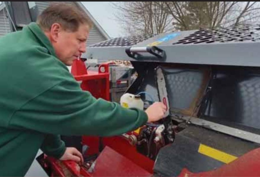
Joe checks the chain tension on the 15-inch cutoff saw. A safety switch shuts down all saw and splitter movement when the cover is open.
