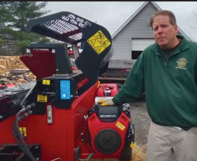
The Japa 365 PRO is self-powered and highway legal for towing. The Honda 690 engine powers the hydraulics for all main functions. Owner Joe Nay estimates that, operating solo, he can process a cord of wood in an hour and a half.
