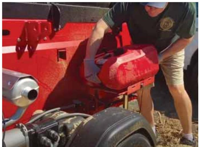
Right: The Japa 365 has a number of thoughtful features, such as a removable fuel tank with a quick coupler.
