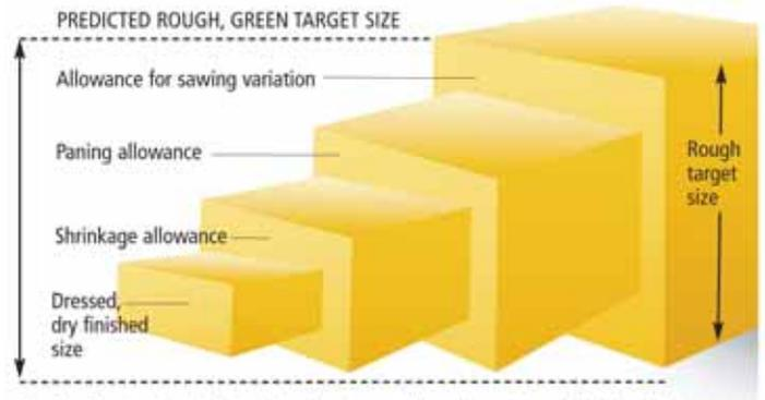
Fig. 3. Factors to determine target lumber size which includes sawing variation.
